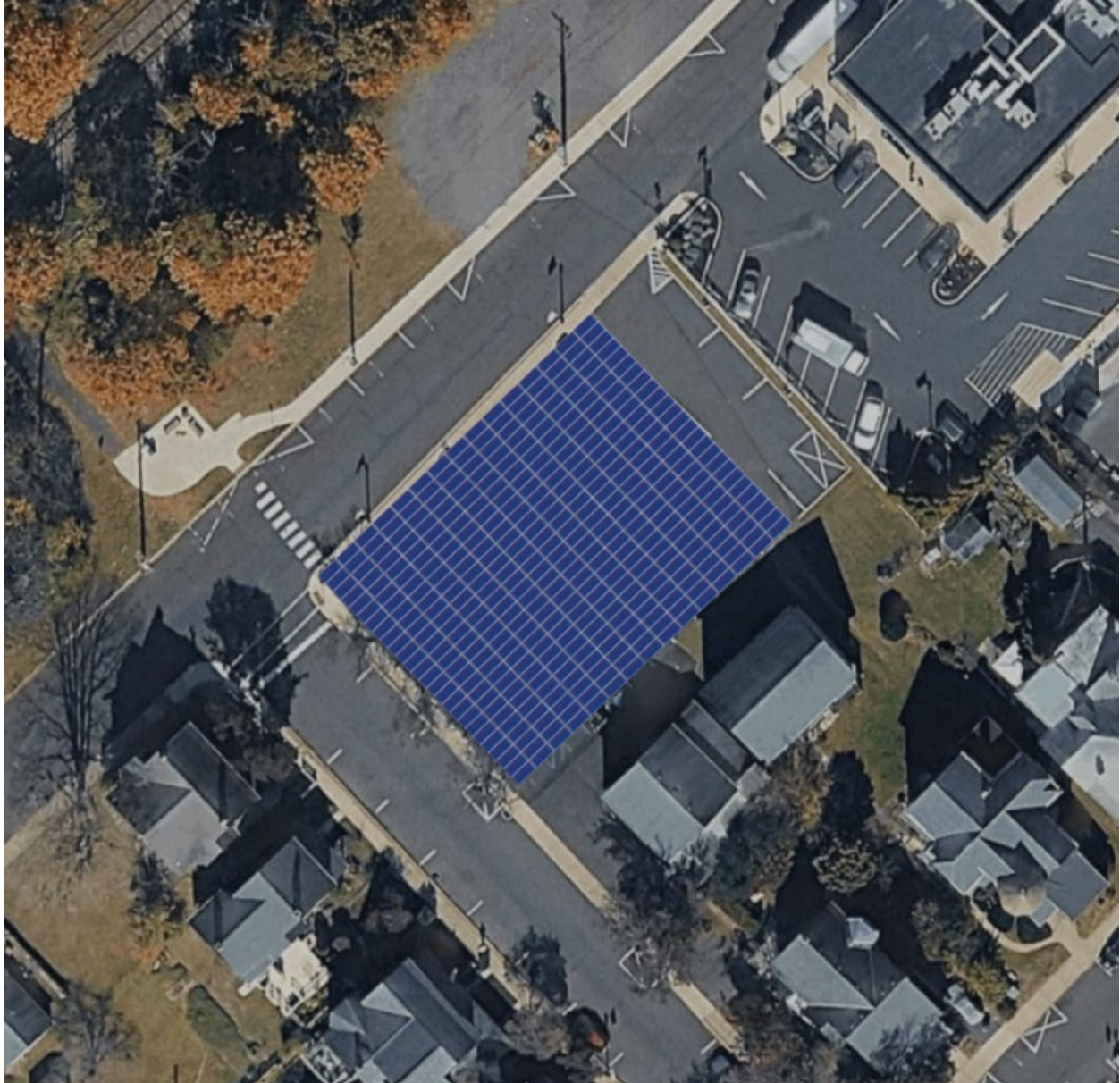
South 7 th Street Parking Lot – 390 PV Modules – 625W/module – 243kWDC total – 200kW worth of inverters
